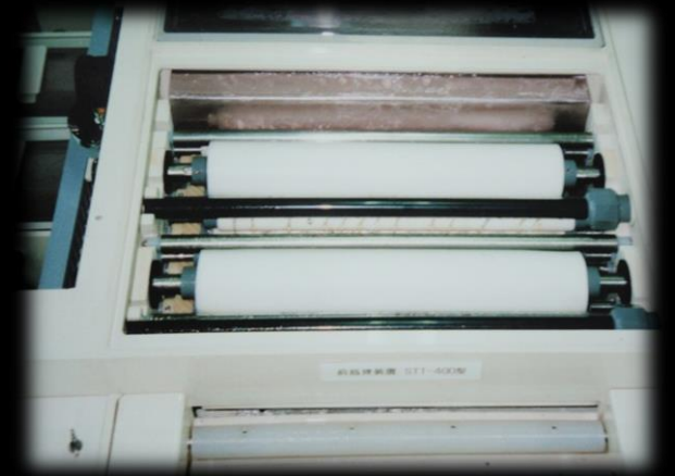
Polishing by PVA Sponge Brush (CaCO 3 is used as Abrasive)
