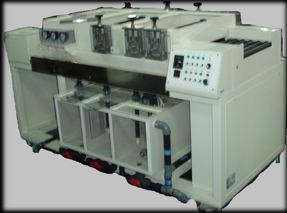
Polishing by PVA Sponge Brush (CaCO 3 is used as Abrasive)
